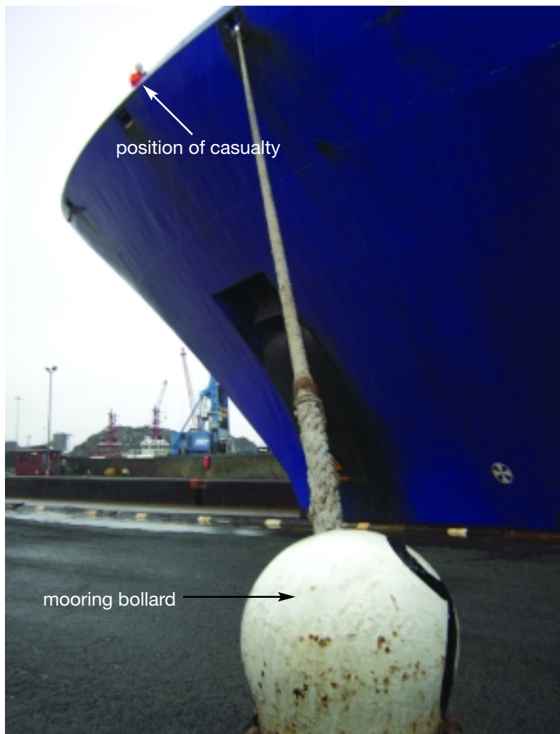
Figure 1: Mooring arrangements at the time of incident
