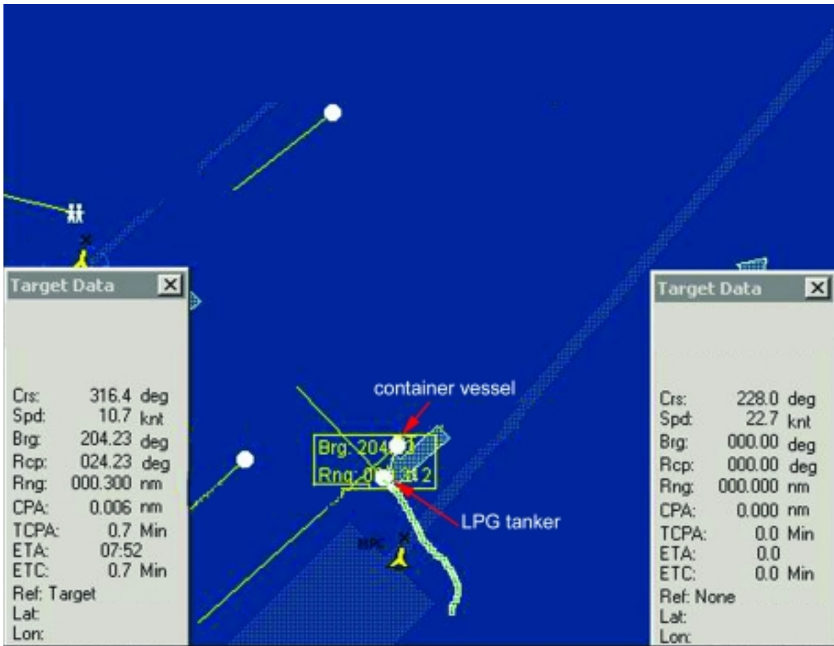
Figure 3: Vessel positions before LPG tanker's turn to port
