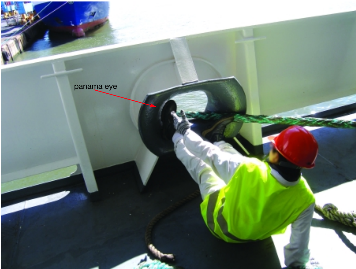
Figure 2: Position of the casualty before being dragged through the panama eye
