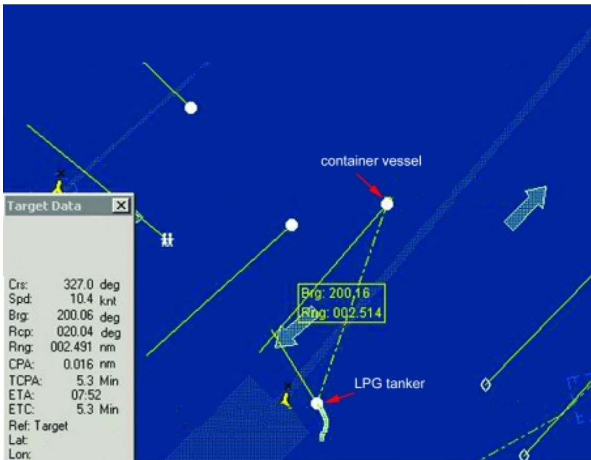
Figure 2: Vessel positions after LPG tanker's change of course
