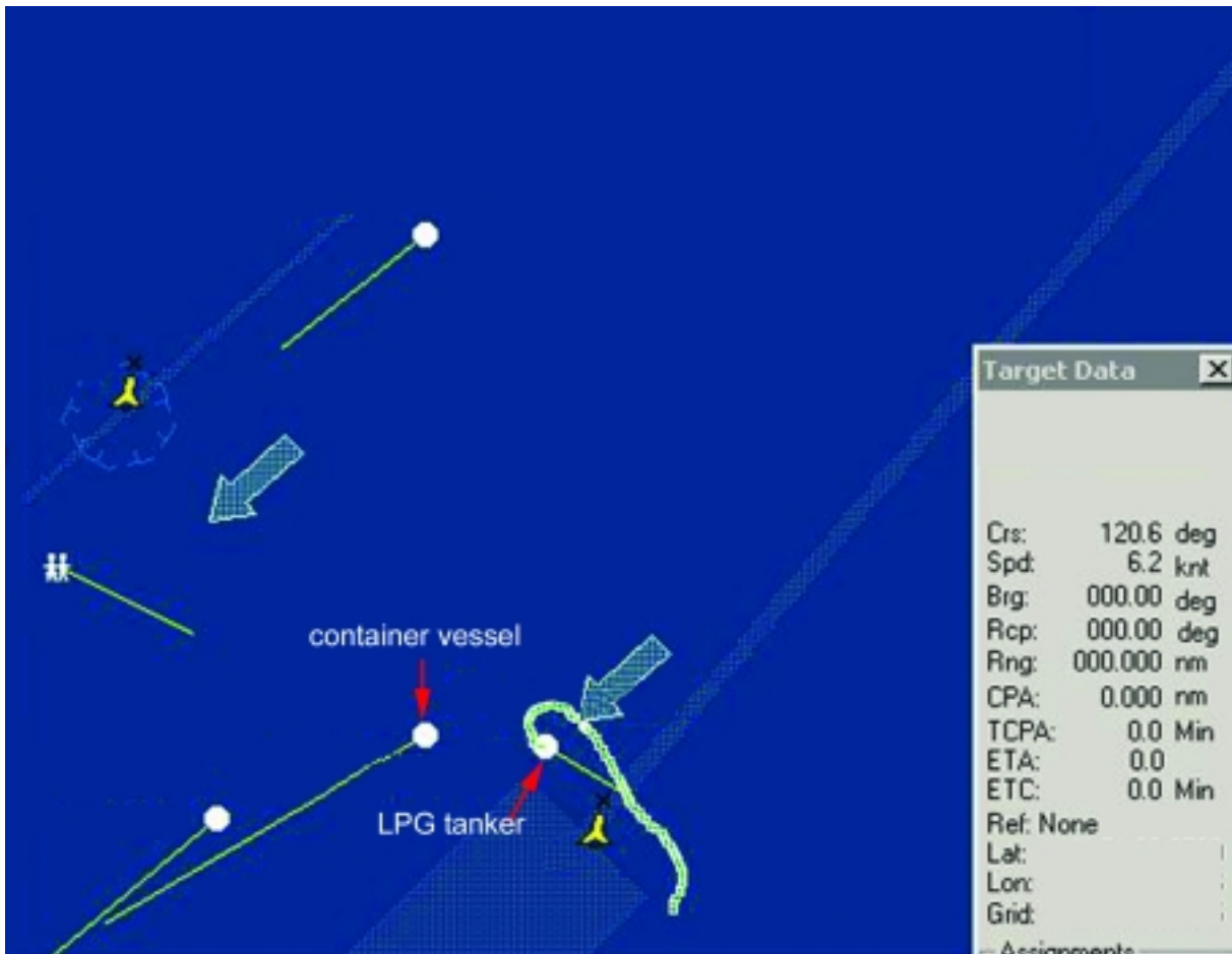
Figure 4: Extent of avoidance action taken by LPG tanker
